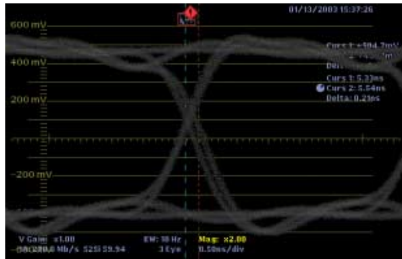
Figure 3-4: Timing Cursors alignment for measuring timing jitter
